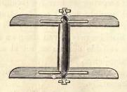
which the explosive force of the combustion of mixed gases is utilized, which explosion expands concertina-like chambers.
